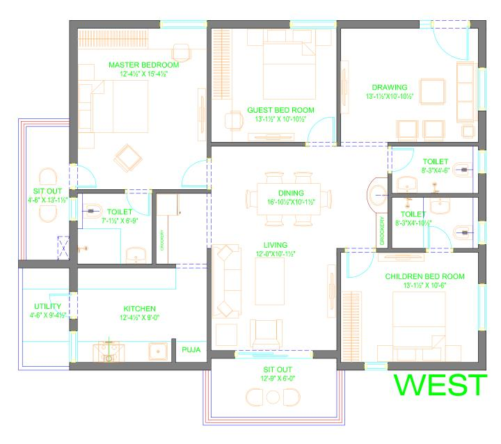
ORIENTATION : FLOOR PLAN CONCEPTUAL- 1 HIGHRISE APARTMENTS FOR AT KOLLUR
